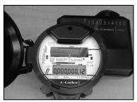
Shine the light on the meter and the reading will appear on the bottom of the two screens. It will flash quickly so you may need to complete this step a couple of times
